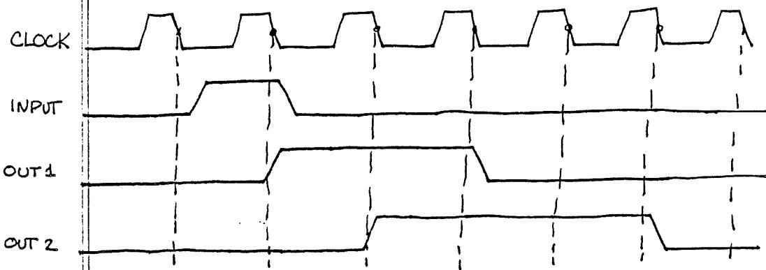
Design two circuits one which takes the given input and produces OUT1. The other takes the given input and produces OUT2.
