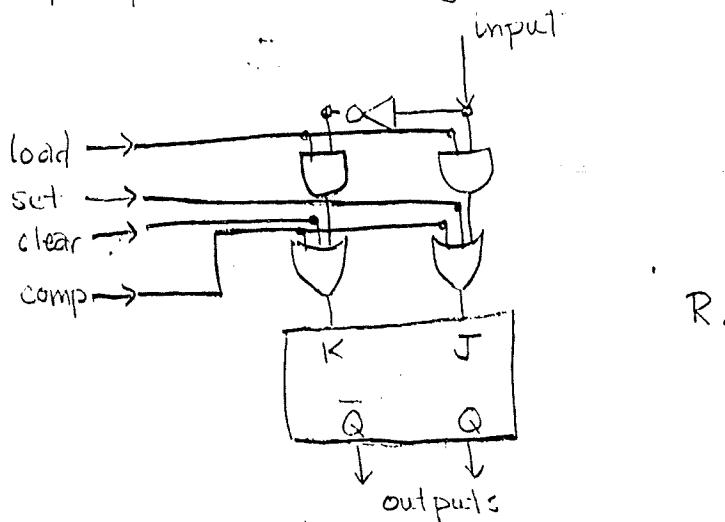
YOUR PROBLEM: WITHOUT putting any gates on the clock line NOR using pre-clear or pre-set, realize the 1-bit register R
