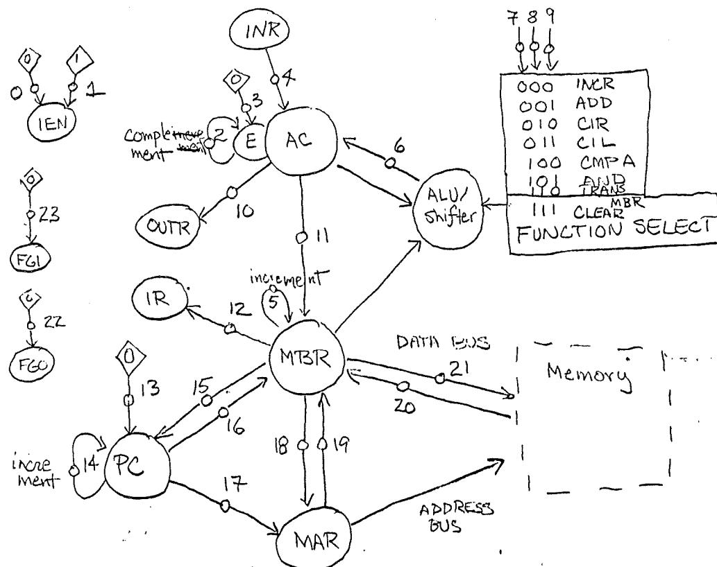
We need a total of 24 "control valves" (which are numbered 0 to 23). Once again we can turn this into a control word which we will write in Hex. Examples
