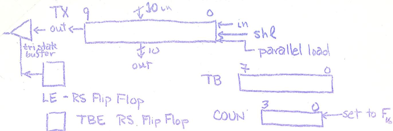
If  $LE = TBE = 0$  then TX (Transmitter) is loaded by  $TX_q \leftarrow 0$  (start bit)  $TX_o \leftarrow 1$  (stop bit) and the contents of TB (Transmit buffer) is put in the middle. At the same time LE (line enable) and TBE (TB empty) are set and COUN (A 4-bit register which is always counting down) is set to  $F_{16}$ .
