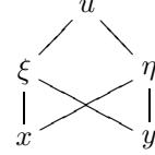
Certainly this is straightforward for this problem as it is a linear equation we get  $\xi = \frac{1}{7}(x + 2y)$  and  $\eta = \frac{1}{7}(2x - 3y)$ . Now we can directly compute  $u_{xx} + u_{yy}$  using the chain rule.
