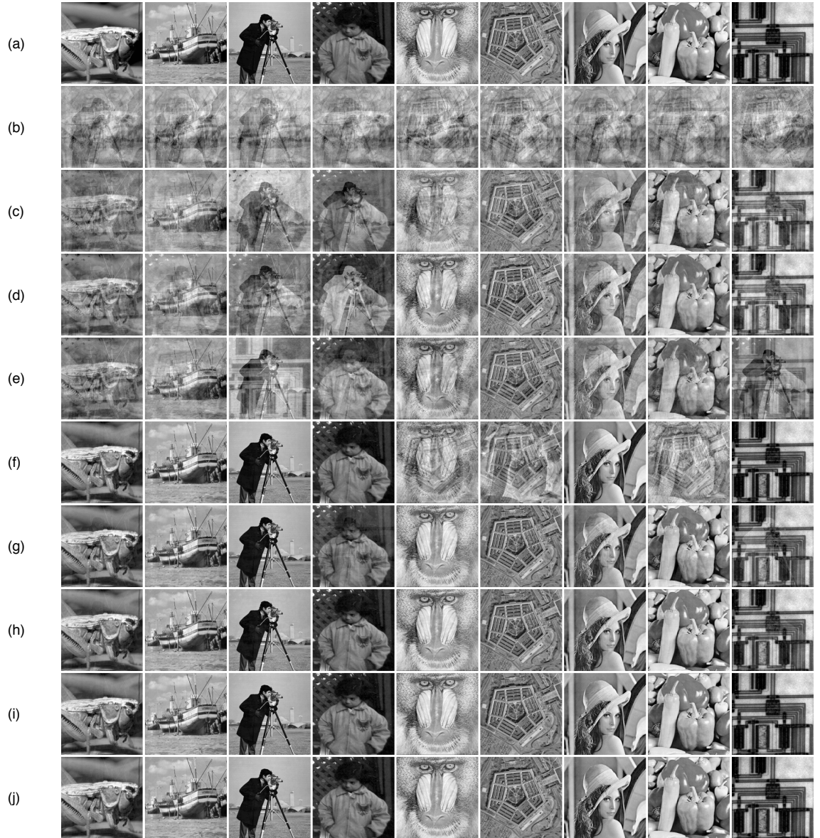
Figure 3: Simulation results using nine natural images of size 200 \times 200 for subjective assessment. (a) Original source images. (b) Mixed images. (c)–(j) Reconstructed sources using the ICA unmixing matrices estimated by the JADE, infomax, fastICA, E-QN-NI, SM-QN-LG, GEKD-ICA, NPICA and OM-QN-VT with RMSE values of 0.191902, 0.196403, 0.213413, 0.128786, 0.065568, 0.041362, 0.030149 and 0.030149, respectively.
