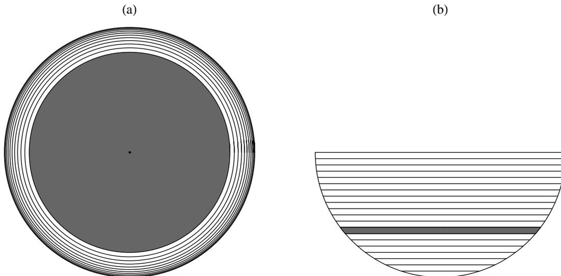
Figure 3: Using coaxial circular disks with sloping rims to partition the volume of liquid in a hemispherical tank. (a) The view from above with a typical elementary volume shaded. (b) Any vertical cross-section through the axis of symmetry, with the same elementary volume shaded.
